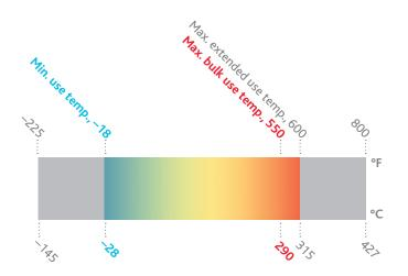
Eastman Therminol<sup>®</sup> SP heat transfer fluid is a unique, synthetic fluid designed to provide reliable, consistent heat transfer performance over a long life at maximum bulk temperatures up to 290°C (550°F).
