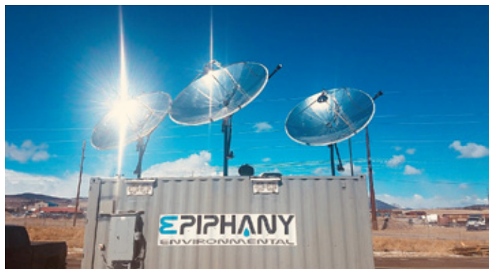
Epiphany designed concentrated solar-powered water purification systems which are now used by the Colorado Department of Transportation.
